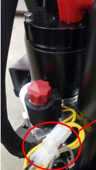
This is plug for drop solenoid valve. Use Multimeter to Measure Whether there is a 24V voltage between grays line & black line when you press the down Button. If yes, it should be the lowering valve body failure, replace it. If there is no voltage. Please measure whether the down button works properly or not.
