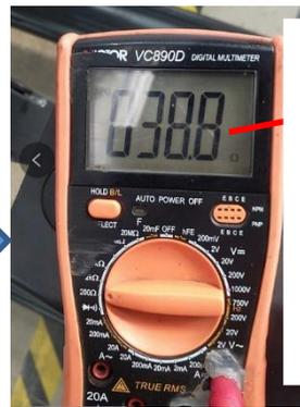
Normally it should be around  $40\ \Omega$  if no Resistance tested. There is a problem with the brake circuit, or the brake coil is short-circuited
