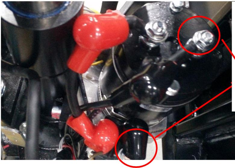
1. Measure the voltage between these two-part shown on the red circle. it is for battery voltage. Check if the voltage normal or not
