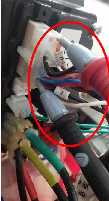
Turn the Multimeter to 24V DC, insert the pin into J1-1(Accelerator 0-5v speed signal)2(Negative). Turn the accelerator after Power-on. And observe whether the Multimeter reading has a linear change of 0-5v voltage
