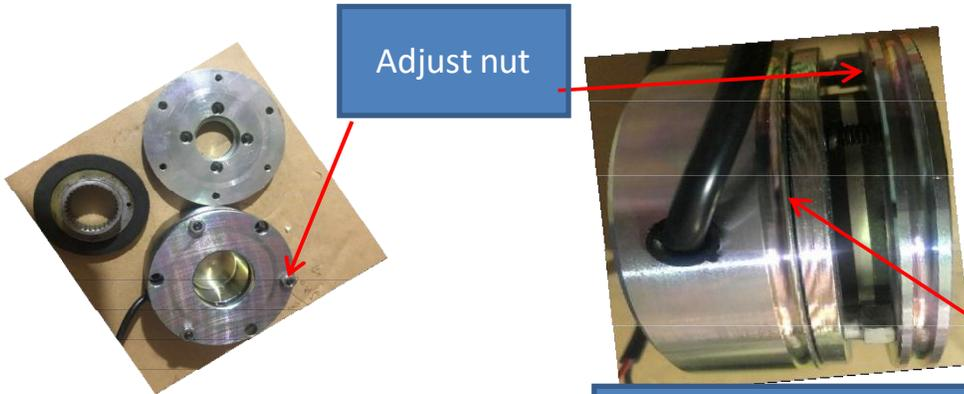
Note: The electromagnetic brake can't be properly connected when it is energized in the free state. It needs to be pulled by external force or installed.
