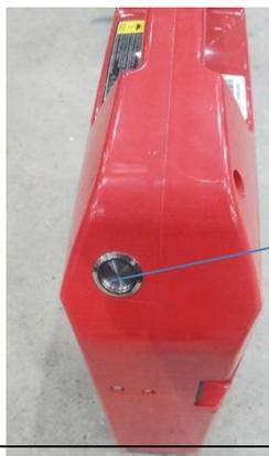
When charging. This switch needs to be turned on. If the battery fails to charge, measure whether the battery voltage is normal.
