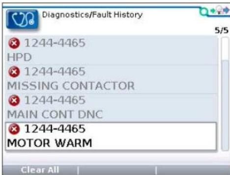
"Clear All" is used to clear the historical fault folder. A function key will only be highlighted when there is a historical fault in the historical fault folder and will be grayed out when there is no historical fault.
