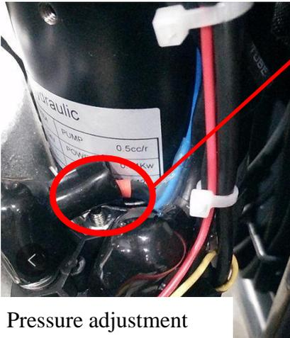
Pressure adjustment valve, note: This valve should not be over-adjusted to avoid deformation of the frame caused by overload.
