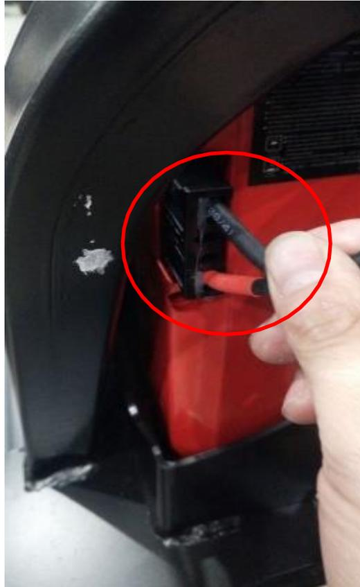
2) Use a Multimeter to measure the voltage of the battery under load
