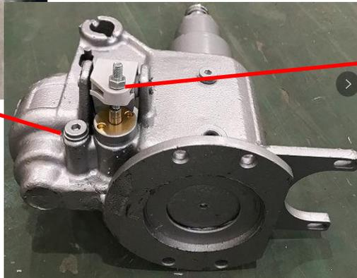
This is a descending valve. If it descends slowly or automatically, adjust the tightness of the descending chain, or check the spool
